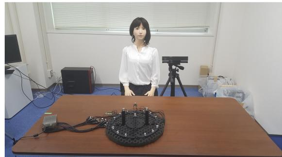
Figure 1: The setup of ERICA's demonstration system, with microphone array and Kinect sensor.
